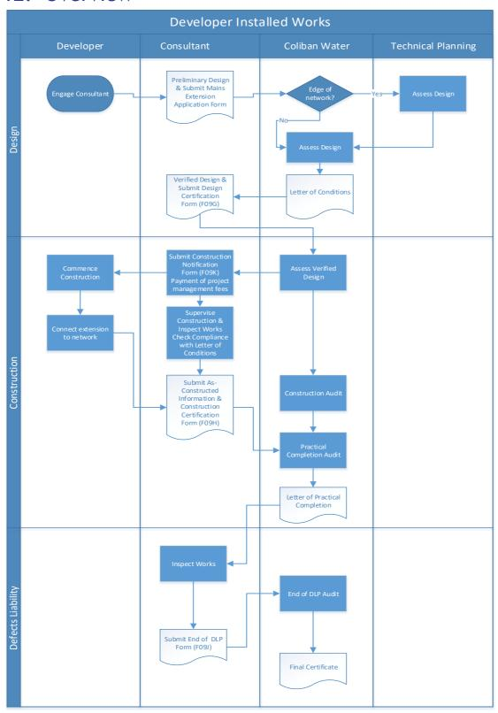
The consultant prepares a preliminary design of the services required to provide water, sewer or recycled water mains to service the proposed development for submission to Coliban Water. They should seek asset plans or concept plans from Coliban Water prior to commencing this preliminary design to establish the most appropriate existing assets to connect to.
